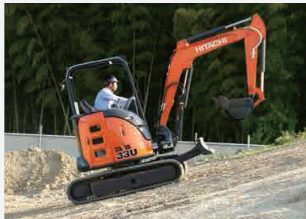
Shown equipped with 1.52 m arm, additional counterweight, armrests and extra piping as optional items.
