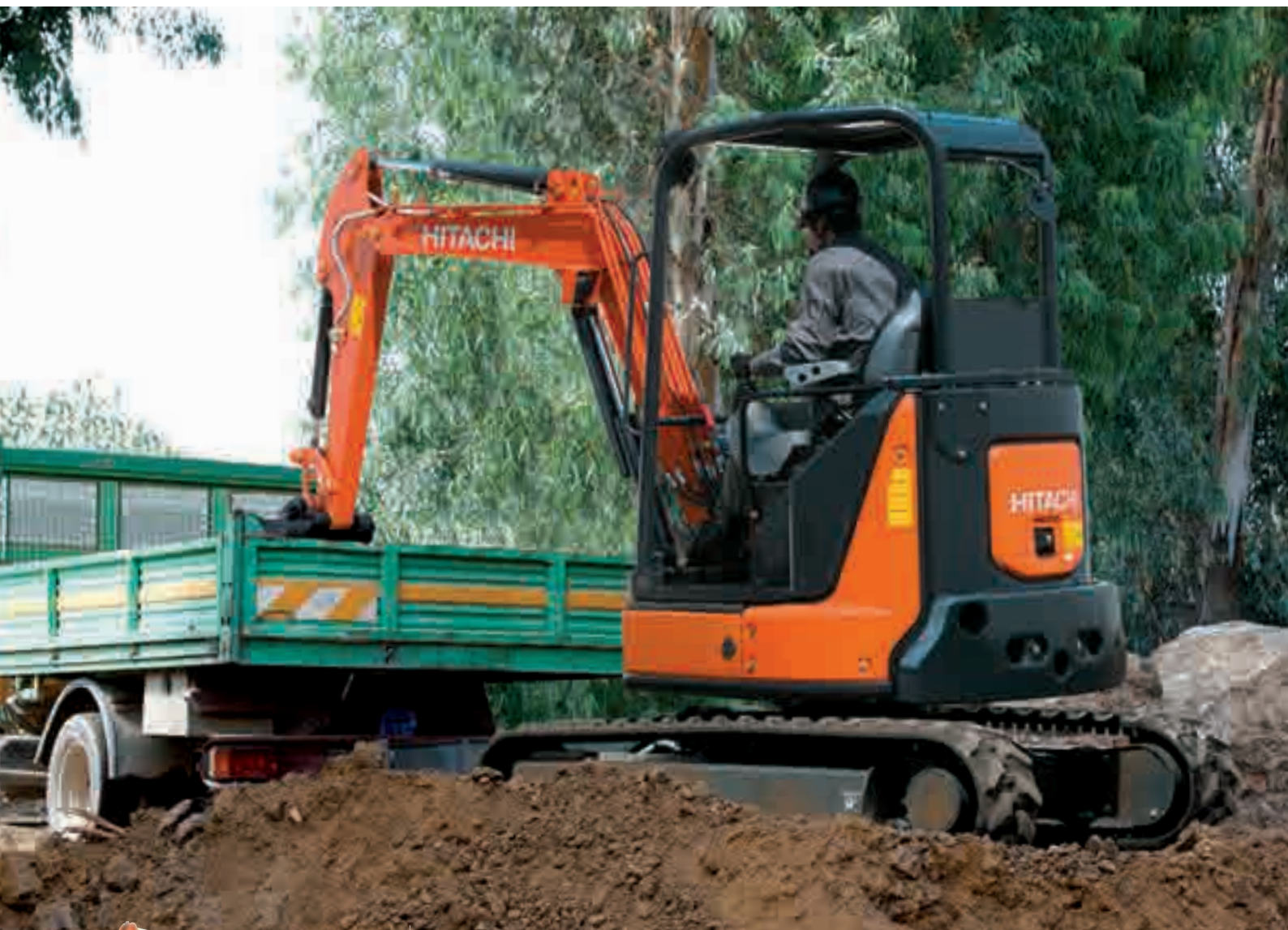
Shown equipped with 1.52 m arm, additional counterweight, armrest and extra piping as optional items.
